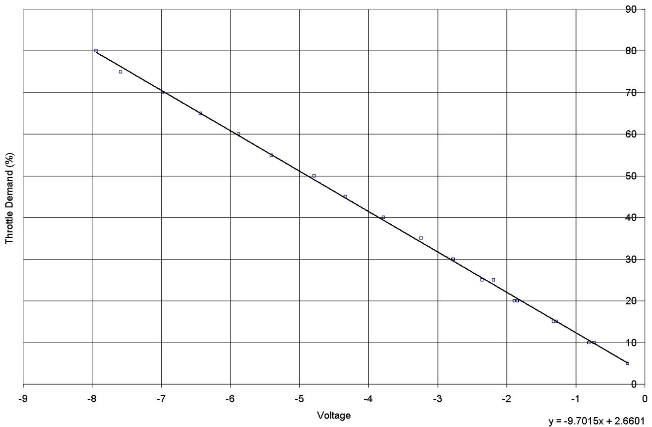
Figure 3.3 – Dynamometer throttle demand calibration
